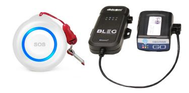
Drivers and workers assigned to a particular vehicle are provided with a key-sized personal (bluetooth) panic button that they can press in case an accident, injury or emergency situation takes place, either from the driver inside the cabin or from a worker outside, at a 50 meters range from the vehicle.
